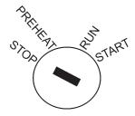
Figure 30. Ignition Switch (OFF)
